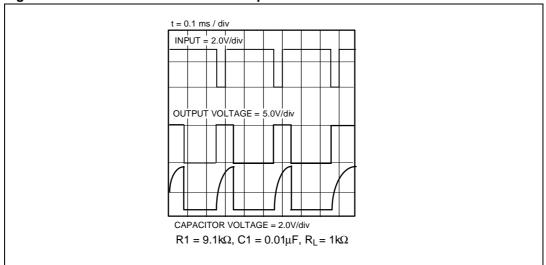
Figure 13. Waveforms in monostable operation
