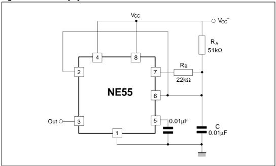
Figure 21. 50% duty cycle oscillator
