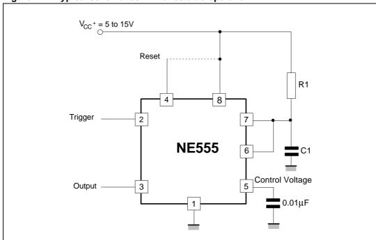
Figure 12. Typical schematics in monostable operation
