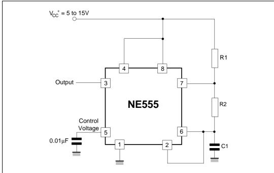
Figure 15. Typical schematics in astable operation
